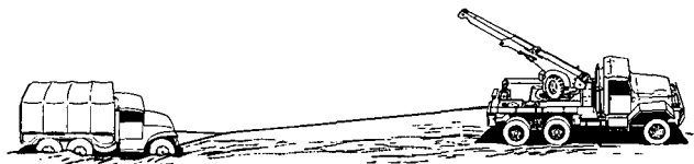
Figure 100. Recovering mired truck with a wrecker truck.
